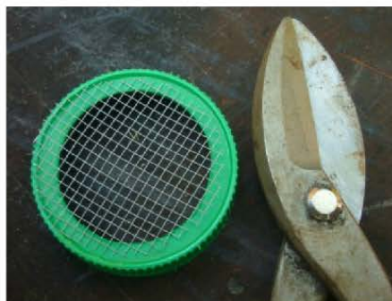
A plastic lid with the inner removed and covered with a section of 1/8" wire mesh. Image courtesy Randy Oliver, www.scientificbeekeeping.com .
