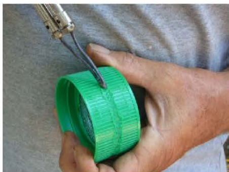
A soldering gun joining the two plastic lids together, with both inner lids removed and the 1/8" wire mesh sandwiched between the lids. Image courtesy Randy Oliver, www.scientificbeekeeping.com .
